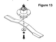
TORQUE BLADE BOLT (LEFT HAND THREADS) TO 85 FT./LBS.
